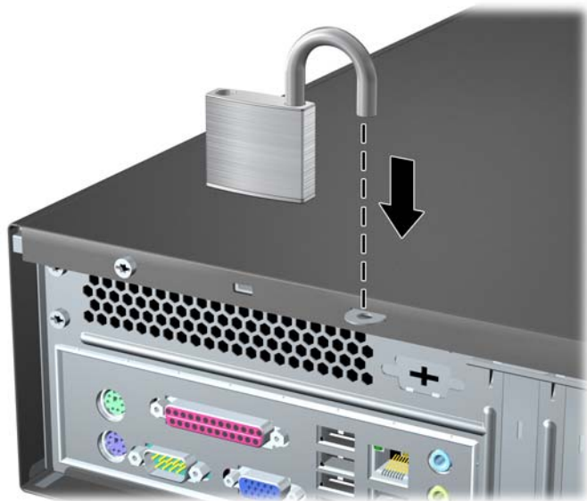
Figure 7-41 Installing a Padlock
